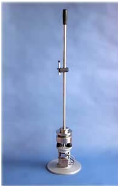
Figure A.9 – Light Weight Deflectometer
