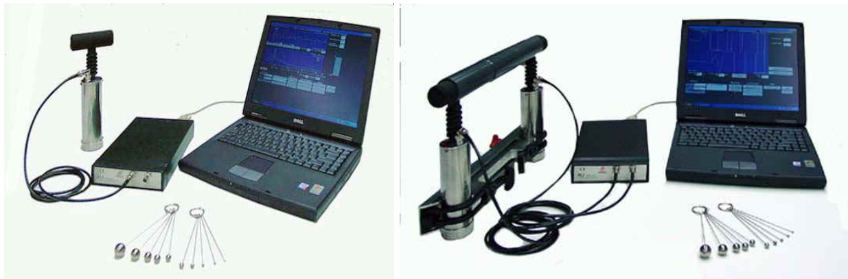
Figure A.20 – Typical Impact Echo Test System
