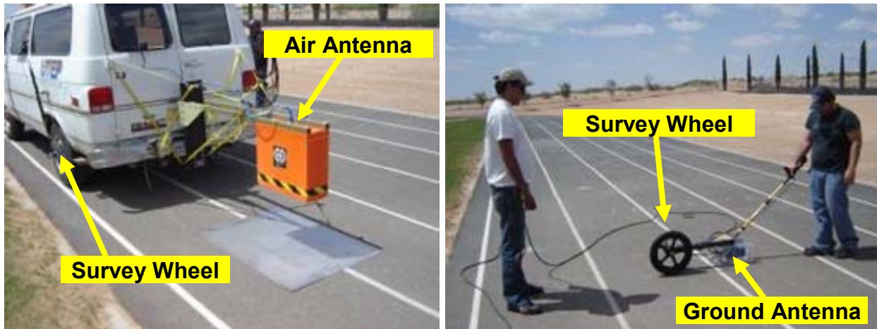
Figure 5.34 – Air Launched (Left) and Ground Coupled (Right) GPR Units
