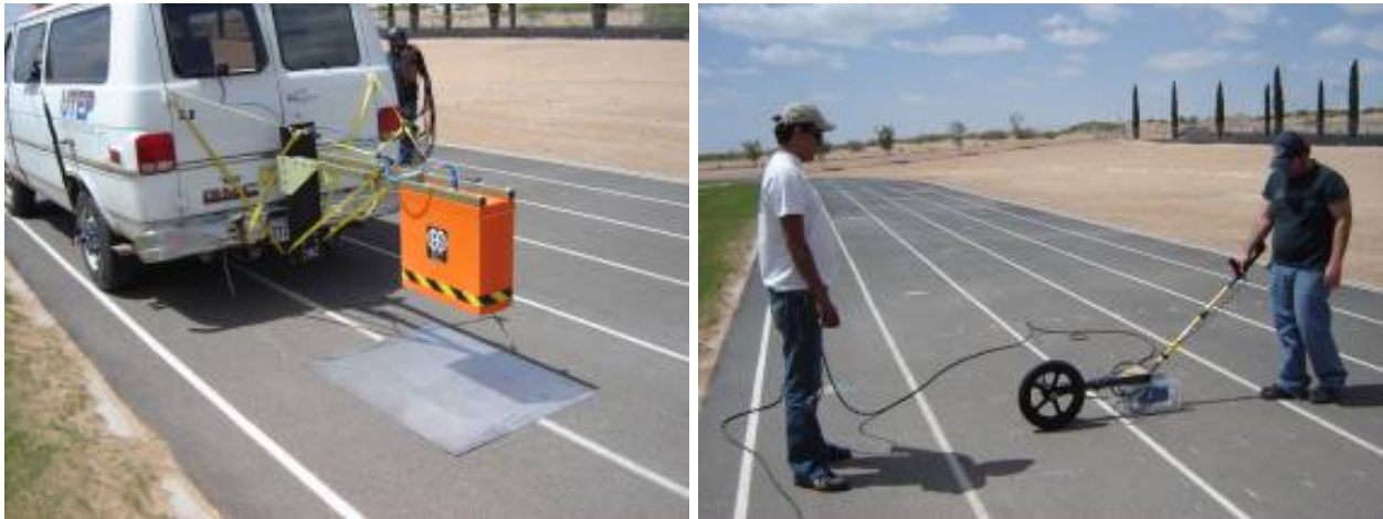
Figure A.1 – Equipment Setup for Air Launched (Left) and Ground Coupled (Right) GPR Units
